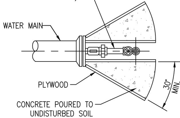
CONCRETE AND PLYWOOD TO HAVE A HEIGHT EQUAL TO THE DIAMETER OF THE PIPE
